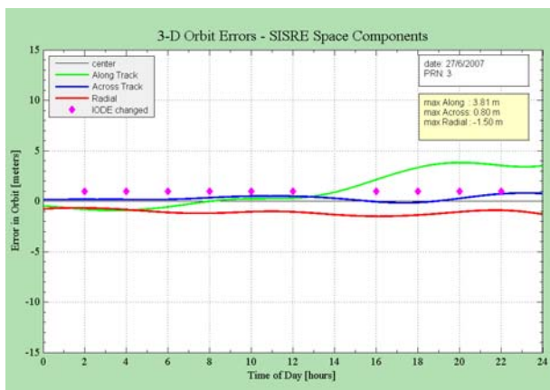
Figure 7: Ephemeris Orbit Errors plot
